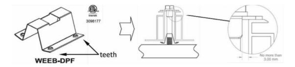
3) Use WEEB-DPF to bond solar modules to module mounting brackets (grounding part is tested to UL467)
