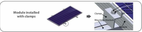
\* The minimum recommended length for each clamp is 50 mm.
