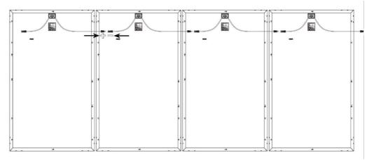
The modules are installed horizontally in the square array, and the module line length: the length of the positive and negative lines is not less than 0.30 m.
